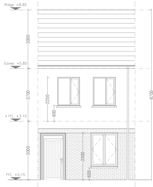
House Type P1 Terraced Front Elevation
